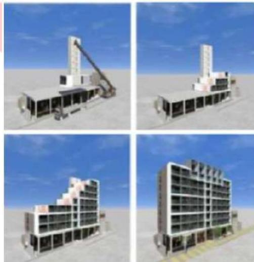
**Gambar 2.20** *PPVC (Prefinished Volumetric Construction)*
