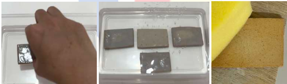
Gambar 4.78 Proses Uji Coba Daya Serap Air ( Sample Tiles )
