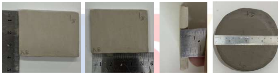
Gambar 4.70 Proses Uji Coba Dimensi ( Bone dry )
