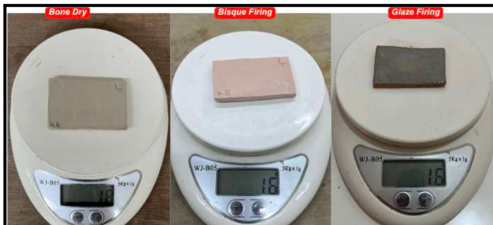
Gambar 4.73 Proses Uji Coba Berat ( Sample Tiles )
