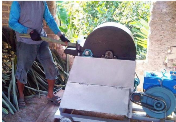
Gambar 2. 19 Mesin Decorticator Sumber: Seratalfiber.com
